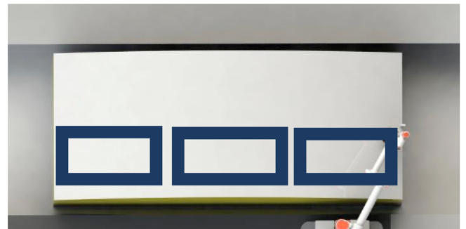
Figure 3: Schematic Diagram of the Rectangular Trajectory.
