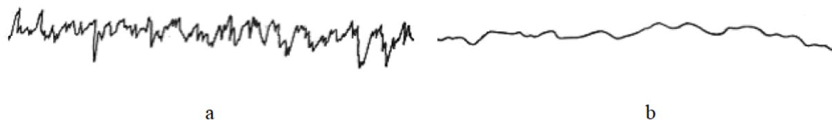
Figure 3: Profilograms of the friction surface of amorphous-crystalline coatings under boundary lubrication conditions with MS-20 oil ( P=15 MPa): a – R_a=0,34\mu\text{m} ( V=0,8 m/s); b – R_a=0,16\mu\text{m} ( V=1,5 m/s); (VUx1000, GUx40).
