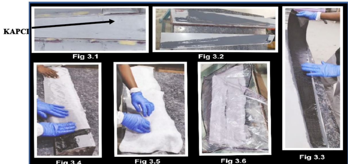
Figure 3: Steps followed in the hand layup technique of fabricating medium density fiber board.
