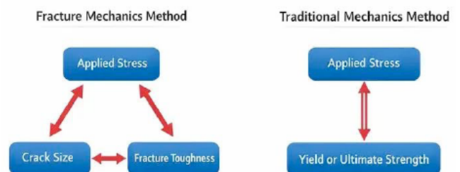
Figure 1: Comparison between the traditional mechanics method and the fracture mechanics method in structural integrity assessment.
