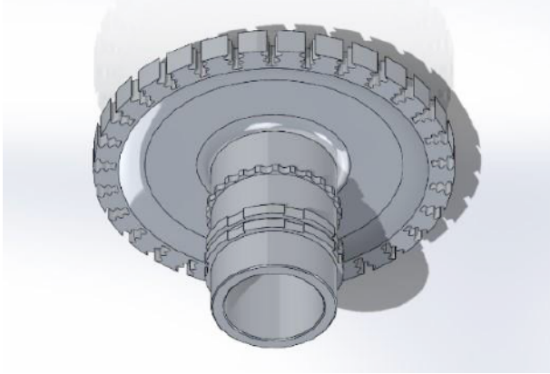
Figure 4: Three-dimensional model of the turbine disc designed in Solid Works in this research.
