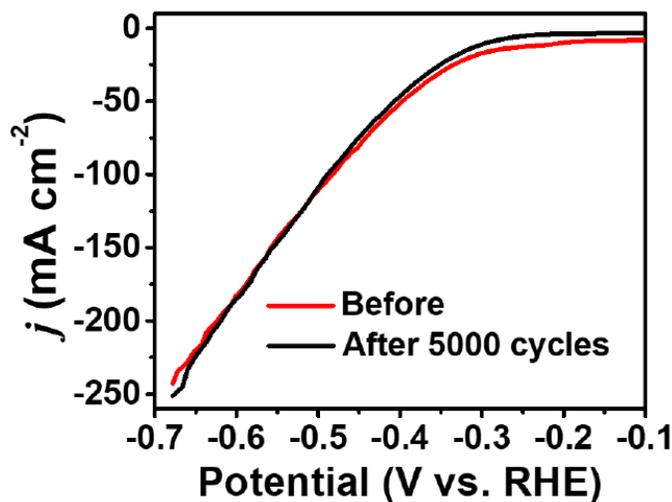
**Figure S17:** LSV curves of NiCoFe-P/CP obtained before and after a durability test. Durability test: 5000 negative LSV scans 0.1 and -0.8 V (vs RHE) at a scan rate of  $100 \text{ mV s}^{-1}$  in 1 M KOH.
