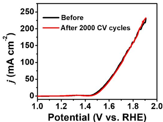
**Figure S14:** LSV curves of NiCoFe-P obtained before and after a durability test. Durability test: 2000 negative LSV scans between 1.2 and 1.7 V (vs RHE) at a scan rate of 100 mV s<sup>-1</sup> in 1 M KOH.
