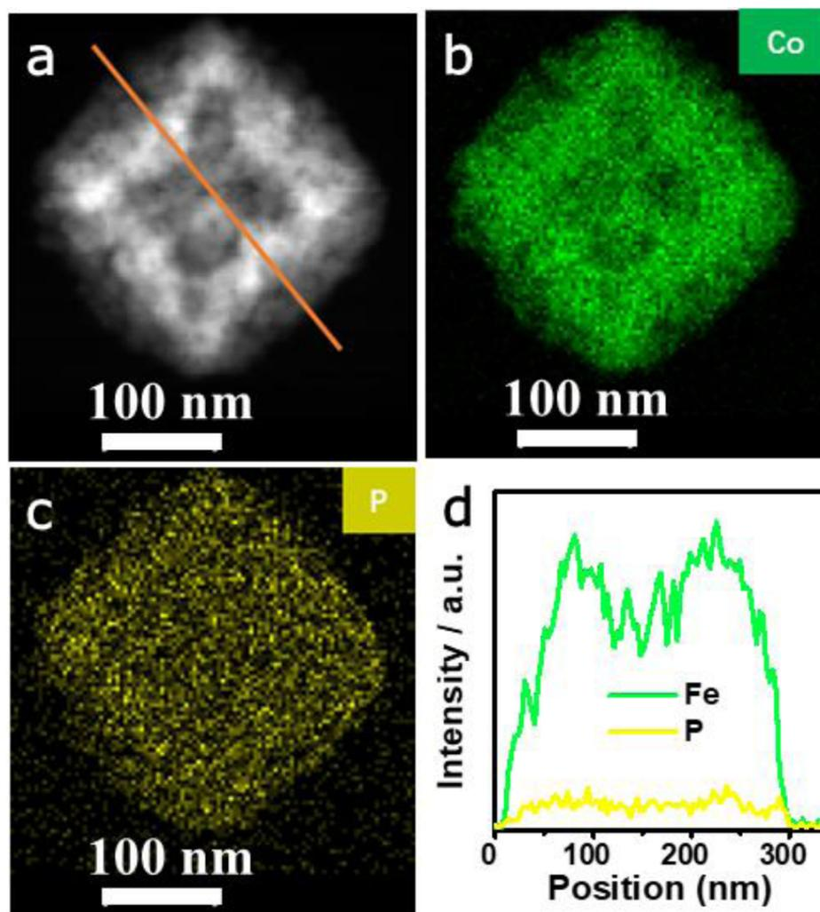
**Figure S8:** (a) Scanning TEM (STEM) image of CoP and the corresponding elemental mapping of (b) Cobalt and (c) Phosphorus. (d) Line-scanning profile of nanostructure of CoP.
