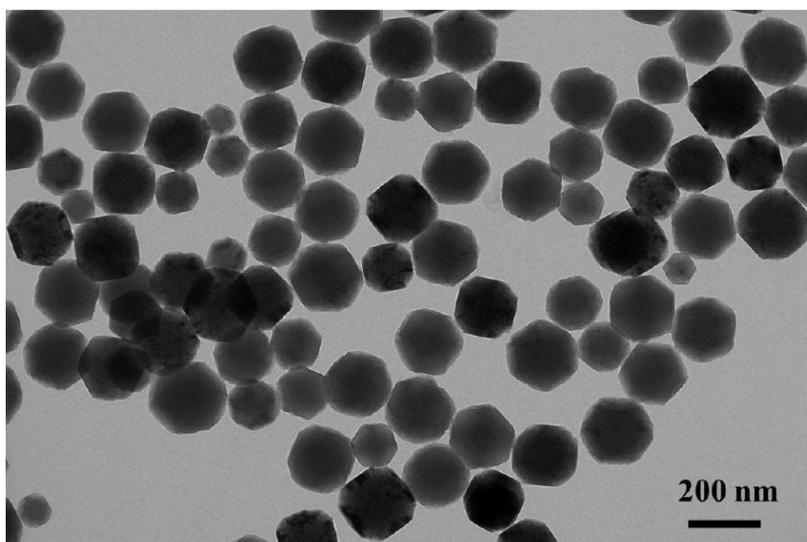
Figure S2: TEM image of the NiCoFe PBA nanostructure.
