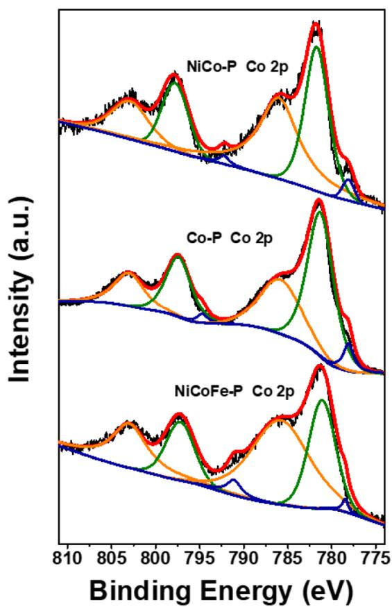
Figure S12: High-resolution XPS spectra of Co 2p of NiCo-P, Co-P and NiCoFe-P.
