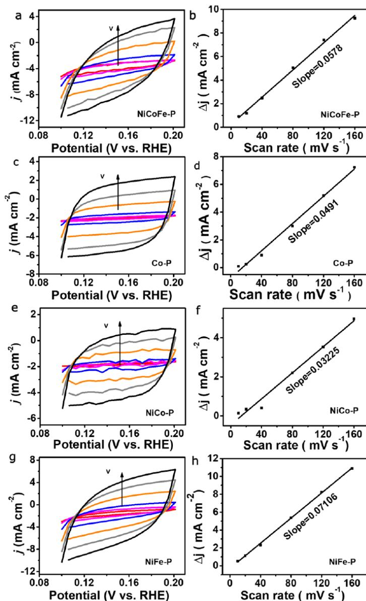
**Figure S15:** (a, c, e and g) electrochemical active surface area analysis by the CV scans in a non-Faradaic potential range of as-prepared electrodes in 1 M KOH for HER at scan rate of  $10 \text{ mV s}^{-1}$ ,  $20 \text{ mV s}^{-1}$ ,  $40 \text{ mV s}^{-1}$ ,  $80 \text{ mV s}^{-1}$ ,  $120 \text{ mV s}^{-1}$  and  $160 \text{ mV s}^{-1}$ . (b, d, f and h) Capacitive current as a function of scan rate.
