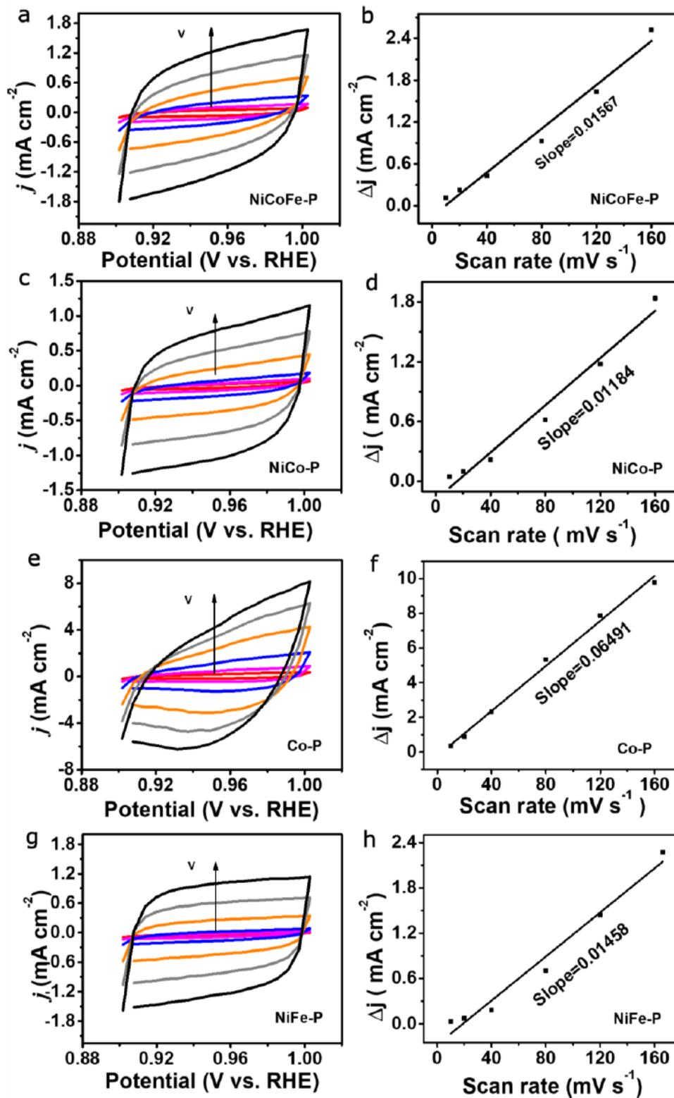
**Figure S16:** (a, c, e and g) electrochemical active surface area analysis by the CV scans in a non-Faradaic potential range of
