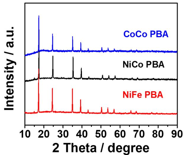
**Figure S4:** Powder X-ray diffraction (XRD) profiles of as-prepared CoCo PBA, NiCo PBA and NiFe PBA.
