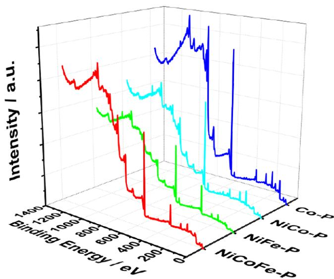
**Figure S9:** XPS survey spectra of NiCoFe-P, NiCo-P, NiFe-P and Co-P.
