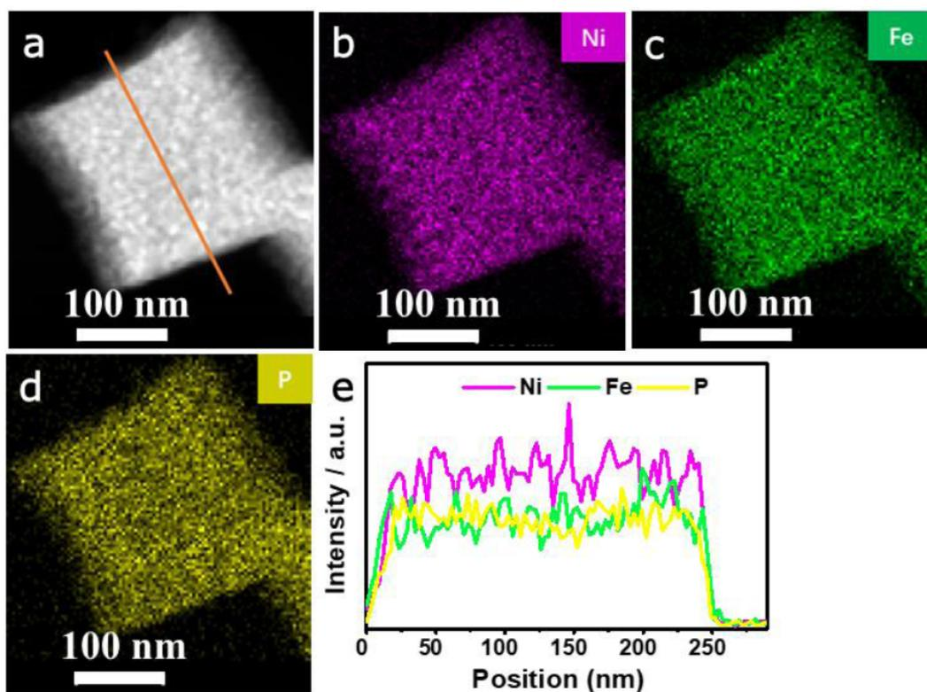
**Figure S7:** (a) Scanning TEM (STEM) image of NiFe-P and the corresponding elemental mapping of (b) Nickel, (c) Iron, and (d) Phosphorus. (e) Line-scanning profile of nanostructure of NiFe-P.
