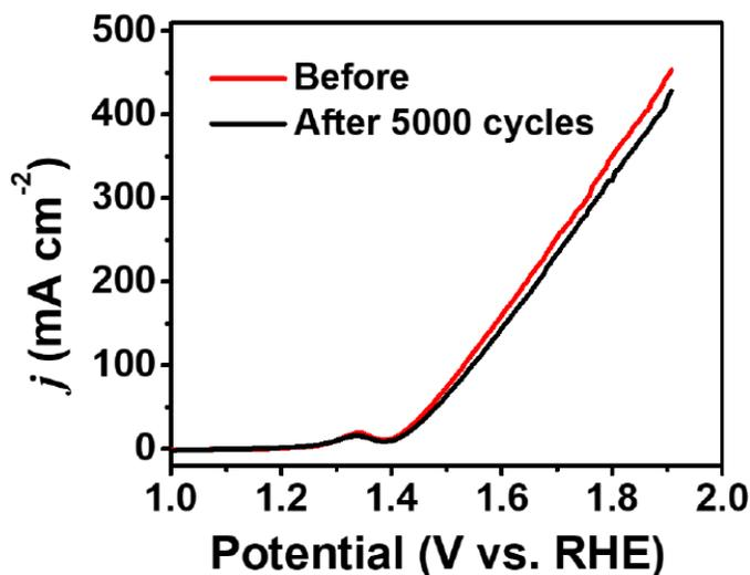
**Figure S18:** LSV curves of NiCoFe-P/CP obtained before and after a durability test. Durability test: 5000 positive LSV scans between 1.2 and 1.7 V (vs RHE) at a scan rate of  $100 \text{ mV s}^{-1}$  in 1 M KOH.
