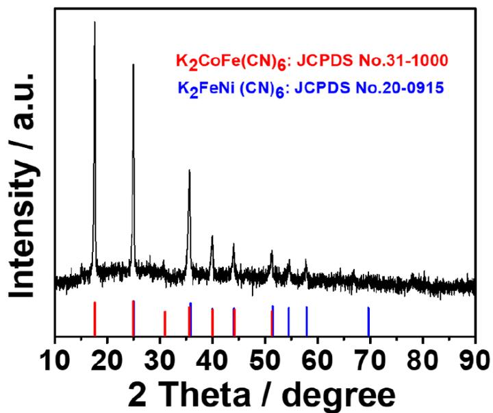
Figure S1: Powder X-ray diffraction (XRD) profiles of as-prepared NiCoFe PBA.
