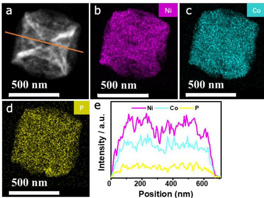
**Figure S6:** (a) Scanning TEM (STEM) image of NiCo-P and the corresponding elemental mapping of (b) Nickel, (c) Cobalt, and (d) Phosphorus. (e) Line-scanning profile of the nanostructure of NiCo-P.
