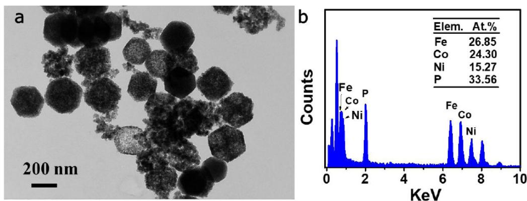
**Figure S3:** (a) TEM image and (b) TEM-EDS spectra of NiCoFe-P.
