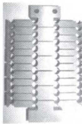
(c) Flexure hinge with a series of 6 layers
