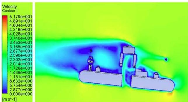
**Figure 7:** Velocity Contour at -5° AoA in Symmetry Plane.
