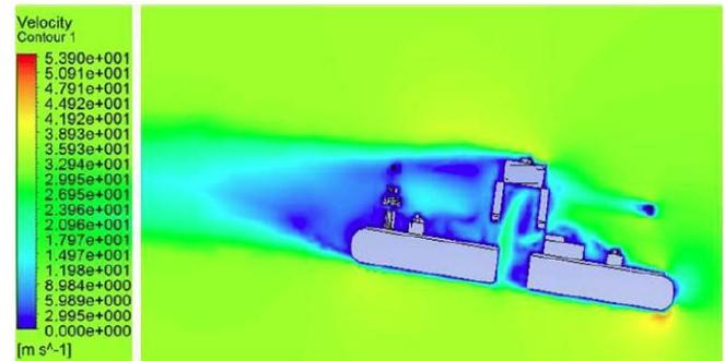
**Figure 8:** Velocity Contour at -8° AoA in Symmetry Plane.
