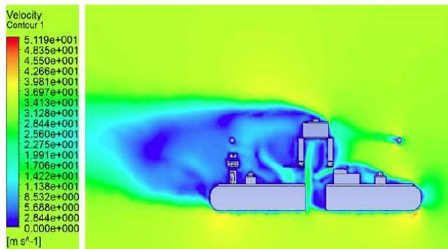
**Figure 6:** Velocity Contour at 0° AoA in Symmetry Plane.
