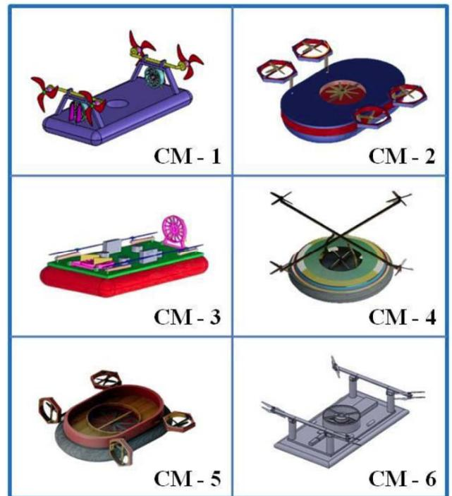
Figure 2: Baseline configurations of UAAV.
