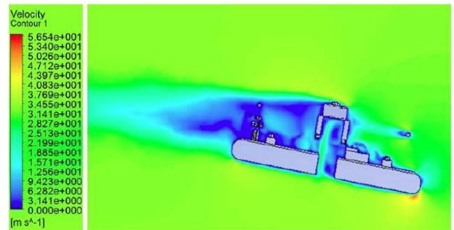
**Figure 9:** Velocity Contour at -10° AoA in Symmetry Plane.
