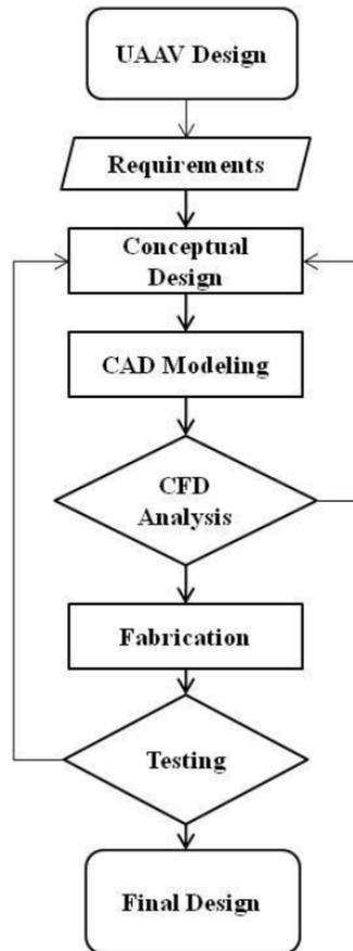
Figure 1: Design methodology of UAAV.
