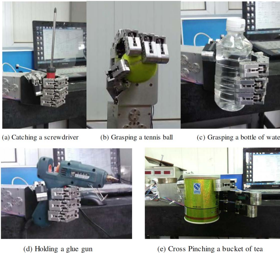
Figure 15: Enveloping grasp of the underactuated four-fingered robot hand prototype.
