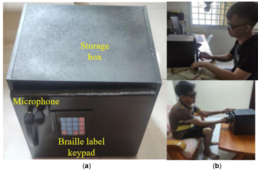
Figure 6: (a) Voice Activated Storage Locker (b) Visual impairment person.
