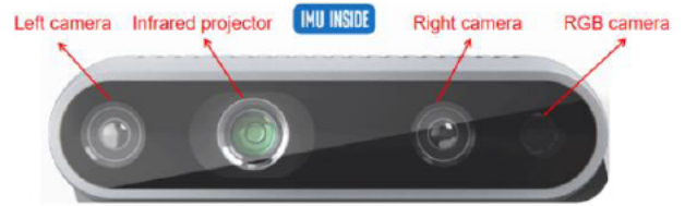
Figure 9: basic structure of Intel real sense d435i.
