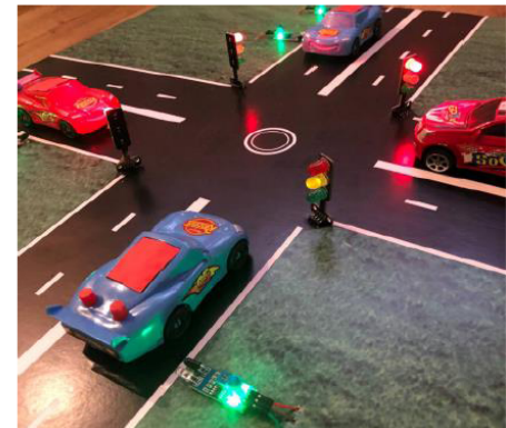
Figure 15: Density-based Traffic Light system response due to equal traffic density in roads.
