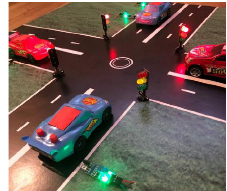
Figure 15: Density-based Traffic Light system response due to equal traffic density in roads.
