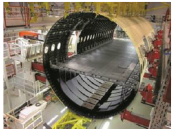
Figure 4: Fuselage section assembly station of A350 XWB [29].
