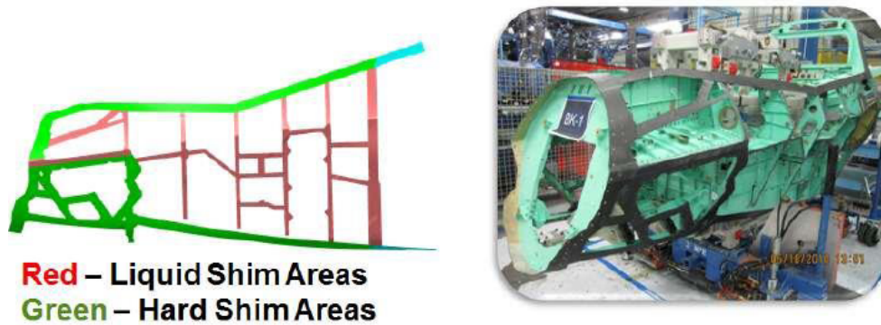
Figure 20: The shimming scheme of F35 forward fuselage [114].
