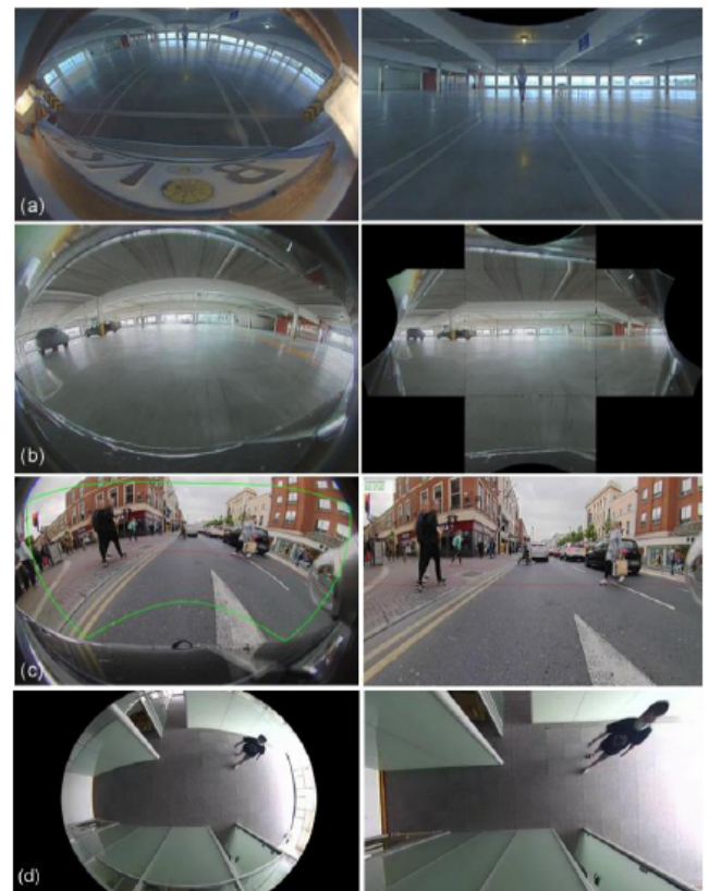
Figure 1: Fisheye images and their calibration [1].
