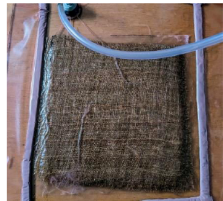
Figure 4: Hand layup assisted vacuum Baggage setup.
