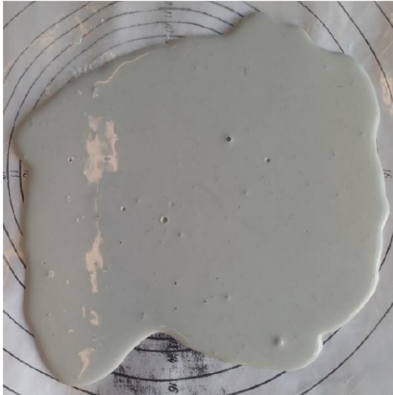
Figure 2: Self-spreading cement dough after the introduction of 0.3% polycarboxylate additive.
