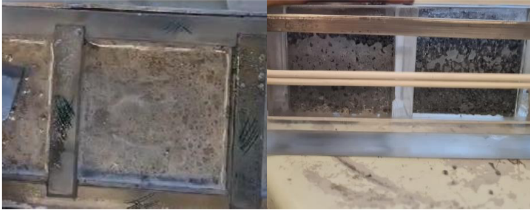
Figure 1: Assessment of the beginning of water separation during the molding process.
